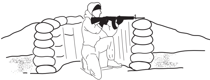
Figure 15-4. Fighting Position Using Sandbags.
