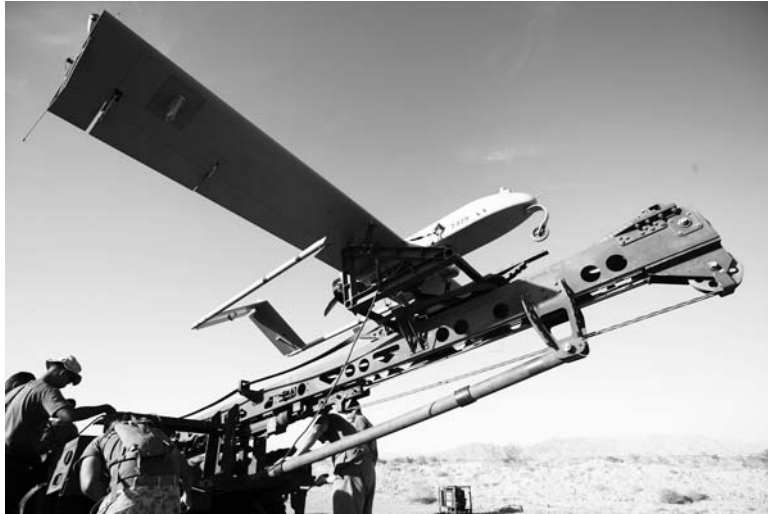
Figure G-3. Shadow Unmanned Aircraft System on Pneumatic Launcher.
