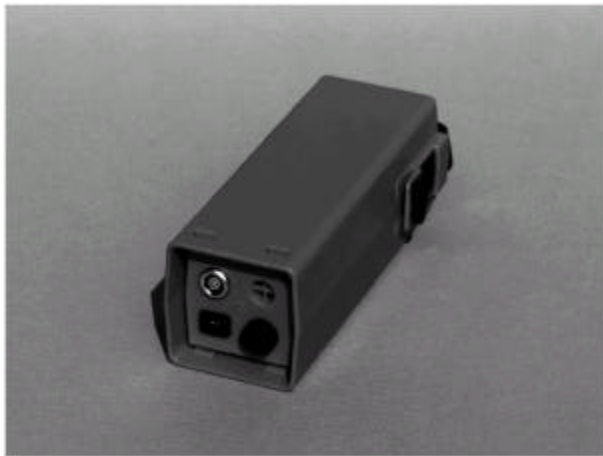
Figure 5-18. GEB-70 NiCad Battery.
