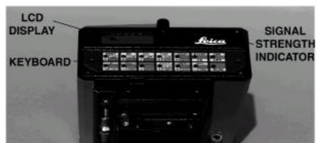
Figure 5-23. DI 3000 Control Panel.
