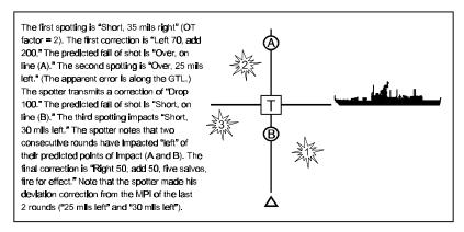
Figure 3-14. Adjustment of Mean Point of Impact.
