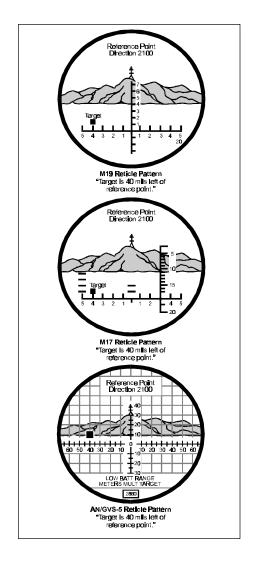
Figure 2-2. Measuring Angular Deviation.
