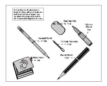
Figure 2-4. Angular Measurement of Common Objects.
