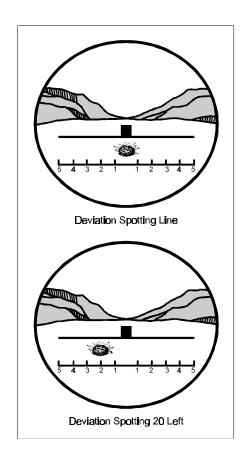
Figure 3-9. Examples of Computing Deviation Spottings.
