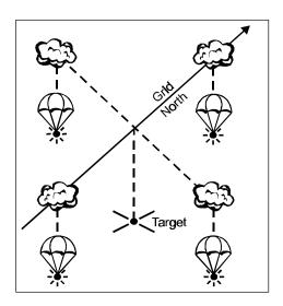
Figure 5-19. Illumination Range and Lateral Spread.
