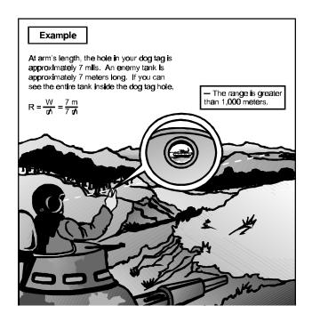
Figure 2-5. Determining Range With Common Objects.
