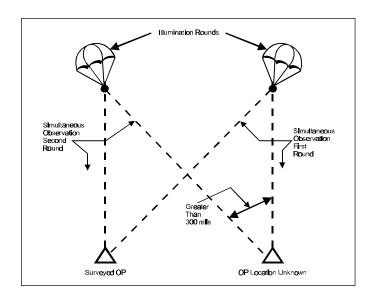
Figure 9-15. Locating Second Observation Point by Simultaneous Observation.
