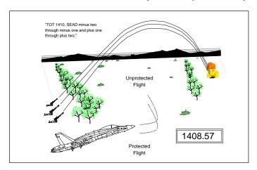
Figure 8-8. Artillery-Close Air Support Aircraft Timed Separation.
