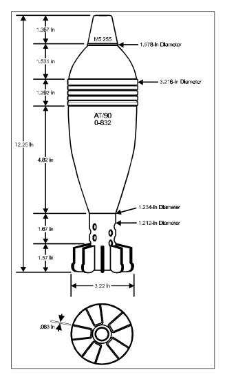
Figure B-12. 82-mm Mortar Round, 5 Fins.
