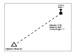
Figure 9-13. Self-Location by Using Resection.
