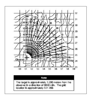
Figure 2-8. Target Location Using the Observed Fire Fan.
