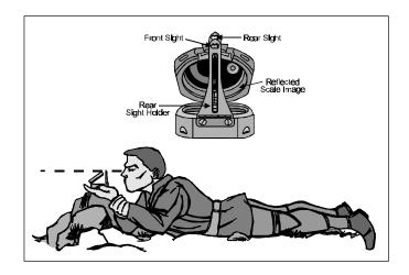
Figure 2-6. Measuring an Azimuth With the M2 Compass.
