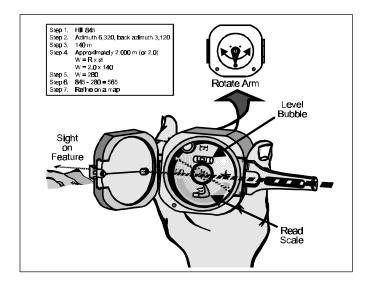
Figure 2-7. Measuring the Vertical Angle.
