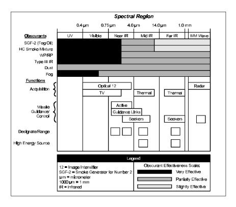
Figure 5-22. Obscurant Effects on Electro-optical Systems.
