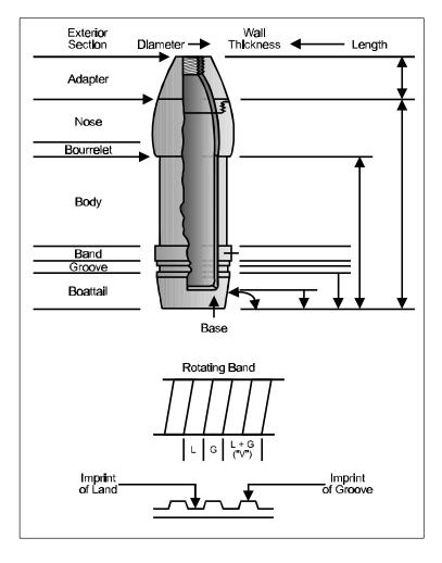
Figure B-7. Typical Shell Showing Critical Measurements.
