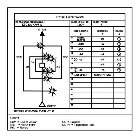
Figure 5-4. Example of Registration Diagram.
