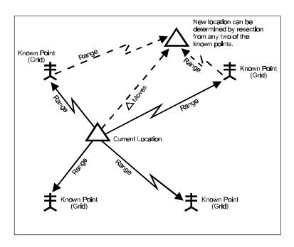
Figure 9-16. Using a Laser To Determine Known Points and New Location.
