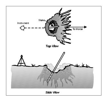
Figure B-6. Fuze Tunnel Method.
