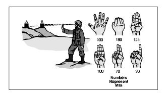
Figure 2-3. Hand Measurement of Angular Deviation.
