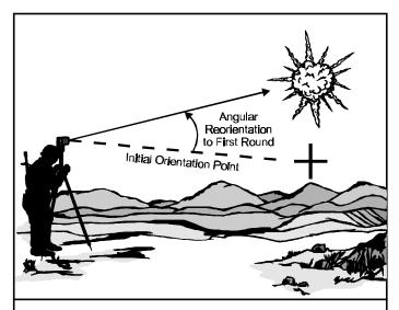
The initial orientation for the FO was "Direction 0430, vertical angle +15." After the burst of 40 mils left of the vertical cross line, the FO determines a direction of 0390. The burst appeared five mils below the horizontal cross line, with a setting on the elevation scales of +15; therefore, the FO obtains a vertical angle of +10. After reporting the instrument readings for the first round, the FO reorients his instrument on a direction of 0390 and a vertical angle of +10.
