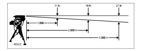
Figure 9-1. Modular Universal Laser Equipment Spot Size.
