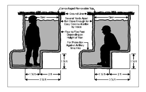
Figure C-2. Observation Post Using One-Man Fighting Holes.
