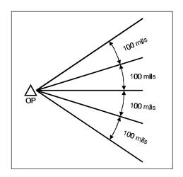
Figure E-2. Radial Lines (Lines of Vision) Ranging Out From the Observation Post.
