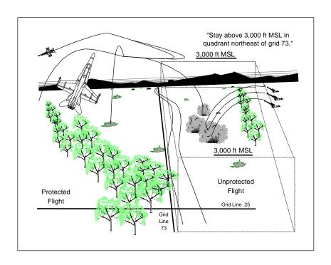
Figure 8-4. Artillery-Close Air Support Aircraft Altitude Separation.
