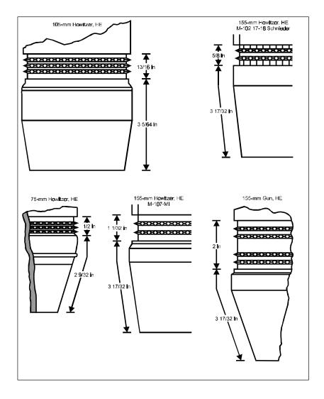
Figure B-8. Shell Fragment Identification, U.S. Ammunition.
