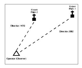
Figure 9-14. Self-Location by Using Triangulation.
