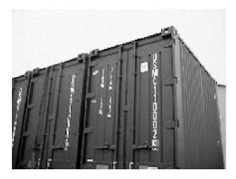
Figure 4-2. QUADCON Markings.
