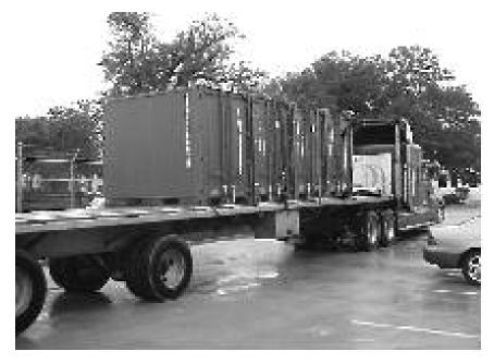
Figure 6-2. Flatbed Trailer with Quadruple Containers.
