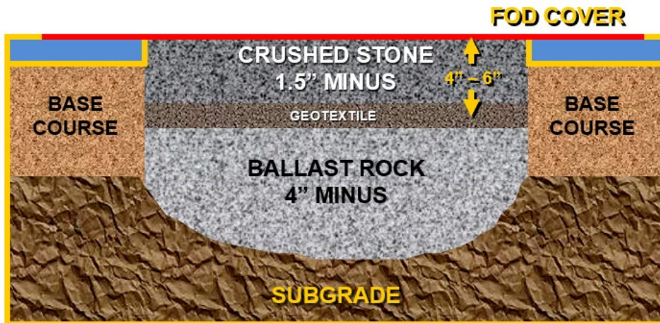
Figure C-12. Choked-ballast Method Layers.
