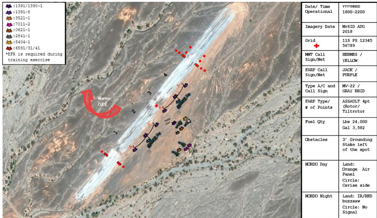
Figure D-1. Notional Assault Forward Arming and Refueling Point Diagram for Rotary-Wing and Tiltrotor Aircraft.
